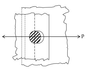
Crushing resistance  $P_C = n.d.t. \sigma_C$
